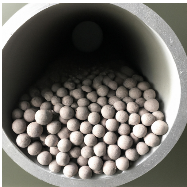
Figure 2. Palladium catalyst (2 - 4 mm spheres) for deoxygenation of hydrogen streams in a tubular fixed-bed reactor.
