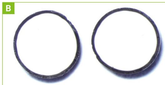
The remarkable performance of ruthenium-based catalyst systems may be attributed to two factors: i) A well-defined distribution of the active material, as is shown in **B** (Ruthenium is primarily located in the outer shell of the pellet), and ii) a narrow nanoparticle size distribution, as is evident in **C**.
