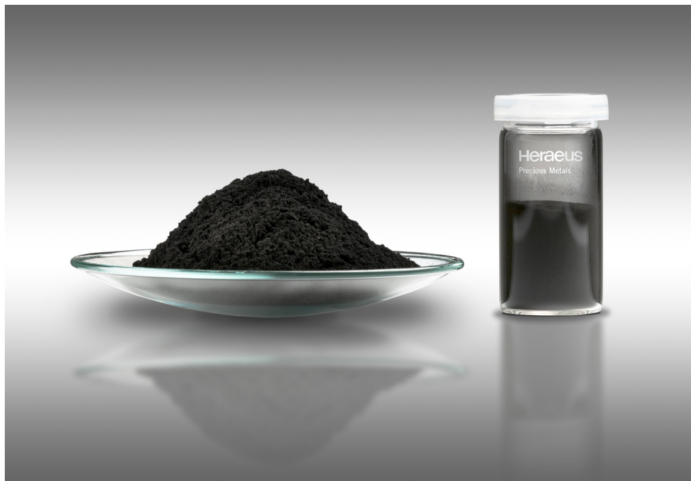
Precious metals catalysts are at the core of an electrolyzer as well as the fuel cell. They catalyze the chemical reactions that are necessary to transfer electrical energy into hydrogen and vice versa.
