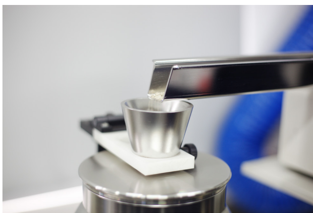
Figure 2. Representative sample splitting for PGM assay (Source: Heraeus Precious Metals).
