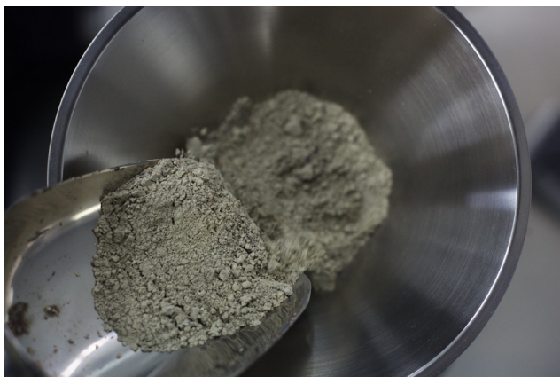
Figure 1. Prepared fine powder for the final sampling stage (Source: Heraeus Precious Metals).
