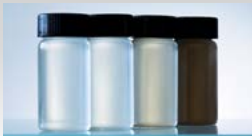
Left: Heat Resistant catalysts before and after stress test (14 d, 50°C storage)
