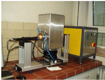
Fig. 2: Contact angle measurement device with high temperature furnace (up to 1700°C)
