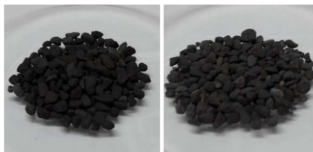
Figure 7. Optical inspection of fresh (left) and aged (right) catalyst
