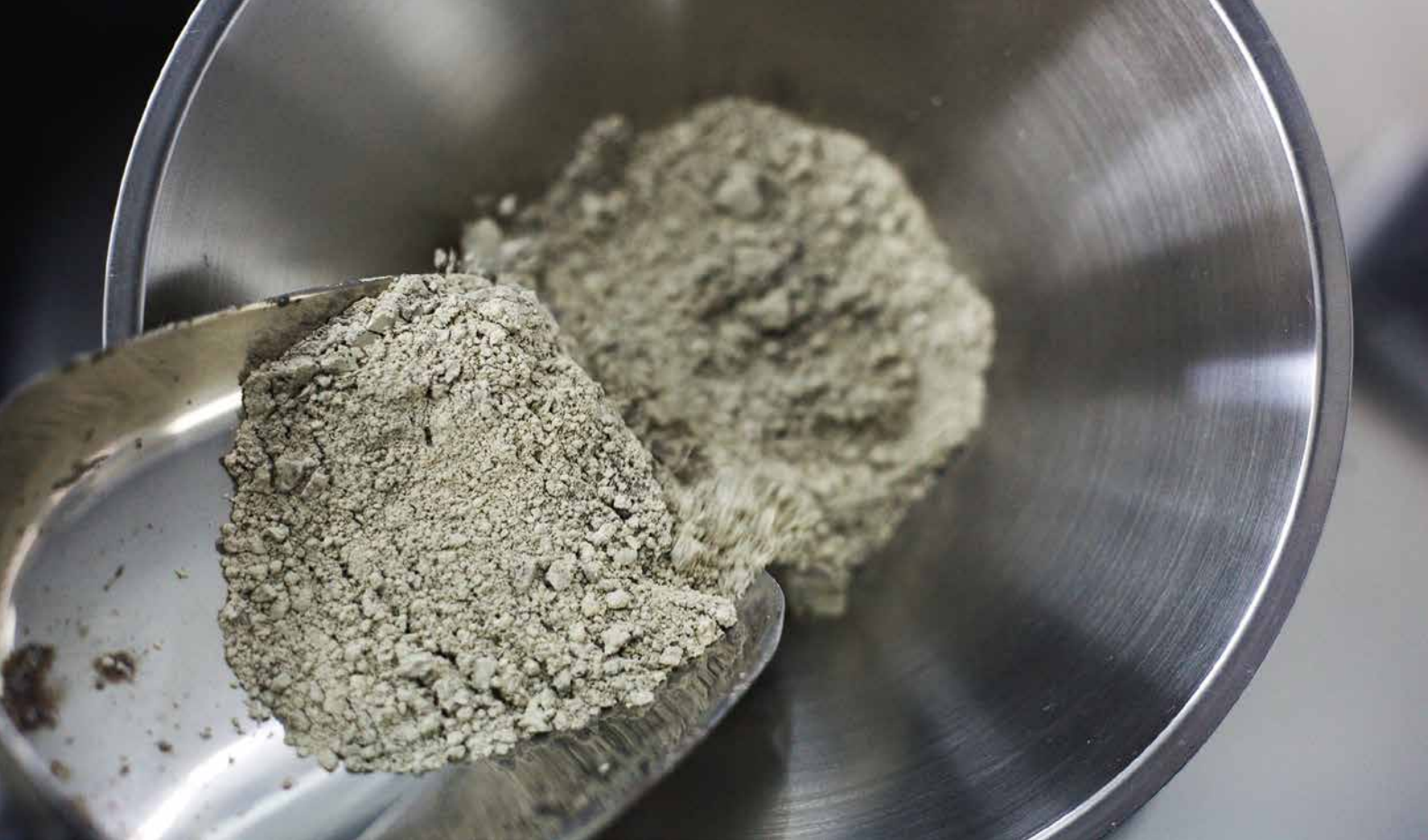
Fig. 4: Platinum-containing material after incineration [Source: Heraeus]
