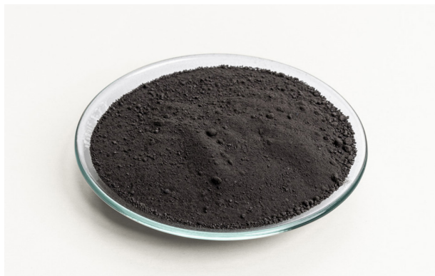
Figure 1. 5%Ru/Al 2 O 3 catalyst for the effective conversion of 5-HMF in DFF.
