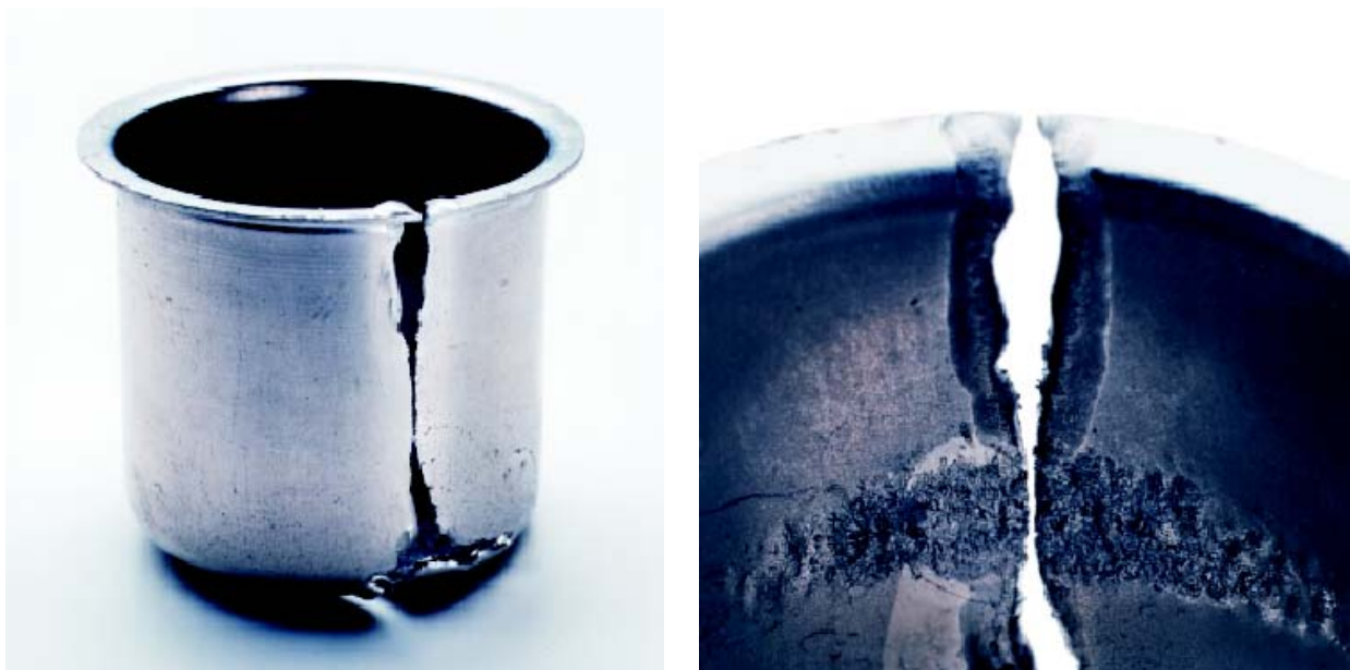
Figure 6 Catastrophic melting of a Pt crucible caused by localised SiC contamination on top rim.
