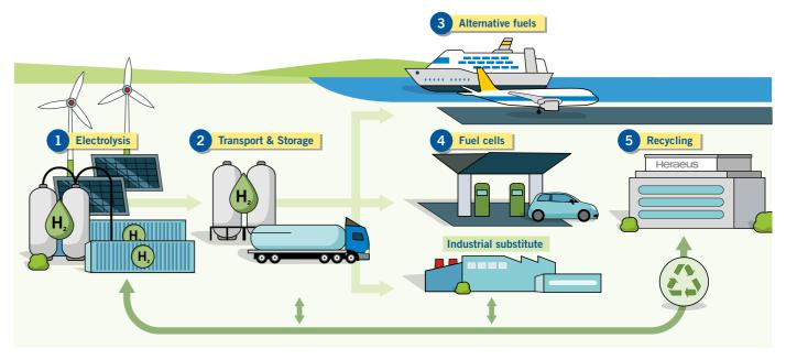
Heraeus supports the hydrogen value chain in many ways: from production via electrolysis (1) and purification, through transport and storage (2), industrial application, for example for the production of alternative fuels (3), and transport-related use as an energy source for fuel cells (4), to precious metal recycling (5).
